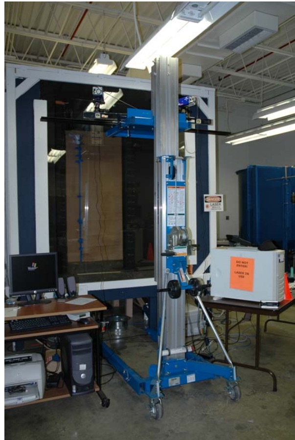
Fig. 2. Photograph of the front of the test cabin showing the lifting mechanism for the stereo cameras.
